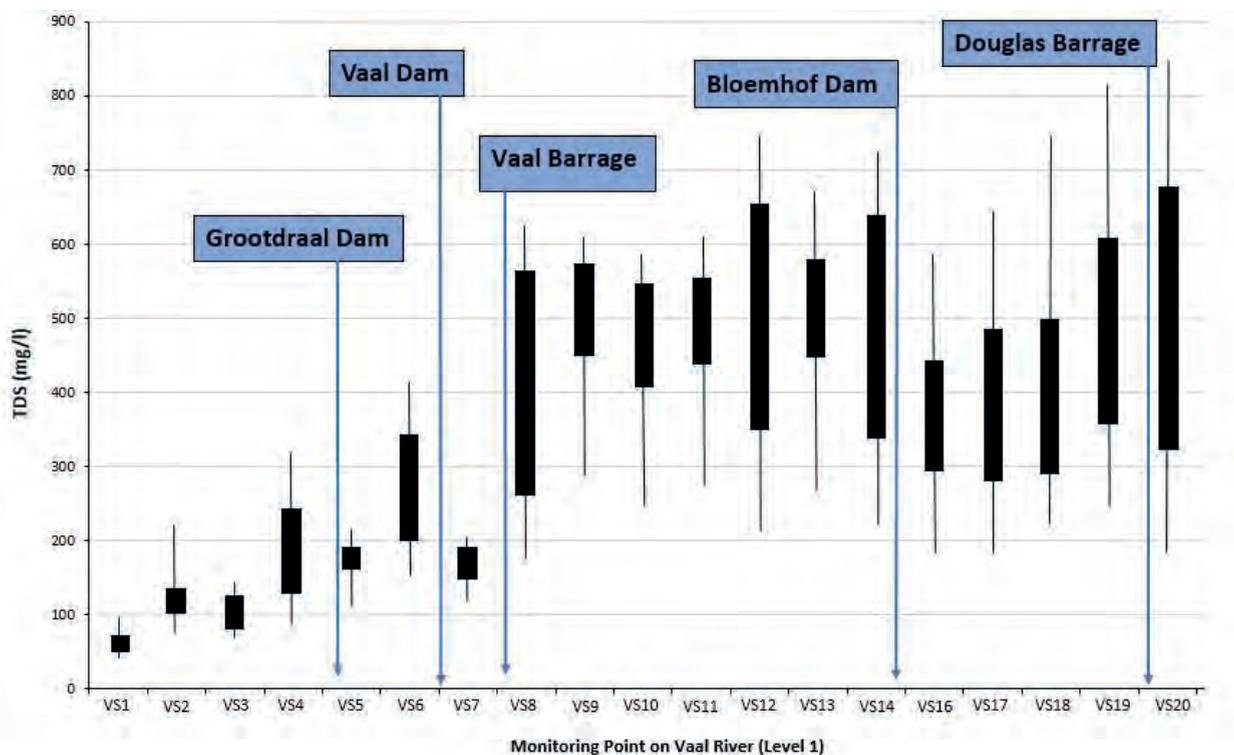
**Figure 4.9:** TDS concentrations (mg/l) in the Vaal River showing the 5<sup>th</sup>, 25<sup>th</sup>, 75<sup>th</sup> and 95<sup>th</sup> TDS concentration percentiles (figure redrawn from DWAF 2008).
